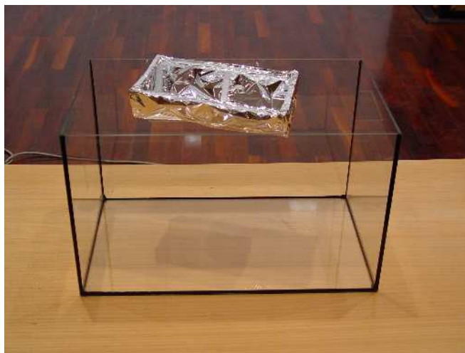
Fig. 1 Aluminium boat floating on sulphur hexafluoride
